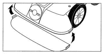
Figure 15: Install the baffle plate.
